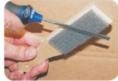
Unload file gullets with the Iron Claw File Cleaning Brush (800-0-1015)
